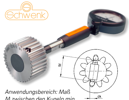
Range of application: Size M min. 10mm to max. 60mm between the balls
