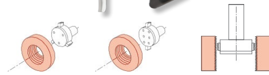
Digital pistol grip bore gauge to measure effective-, pitch and major diameter between M4 – 300mm / No. 8 UN – 12".
