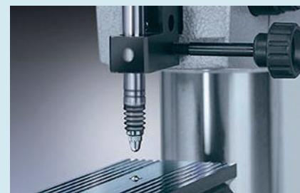
Difference measurements with opposite polarity signs (+A -B)
