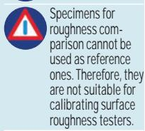
Specimens for roughness comparison cannot be used as reference ones. Therefore, they are not suitable for calibrating surface roughness testers.
