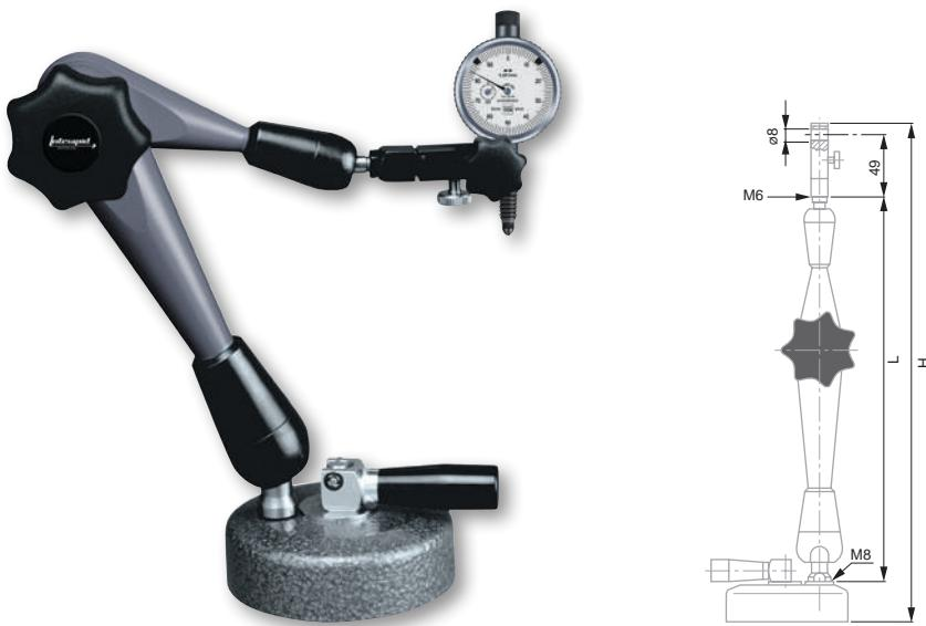
**A** Round suction base made of aluminium ( $\varnothing$  88 mm, height 28 mm) with flat suction base. Articulations made from duralumin. Suction controlled by lever switch. Dovetail clamp with an  $\varnothing$  8 mm clamping bore.
