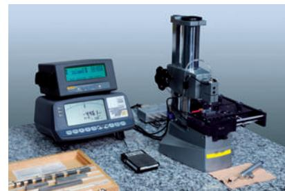
If specified, TESA can also provide the temperature device available as an option. This device has 4 PT100 platinum resistances, each capturing the temperature of the two gauge blocks along with that of both the measuring table and the support. Computer-aided data processing lets you carry out any calibration most reliably and rationally – for sure.
