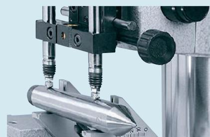
Establishing form and position errors with "max - min" memory function as in the example for runout errors
