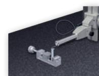
RUGOSURF 90G in profile measuring mode with PROFILE SET 2 mm
