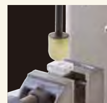
The switch feeling test with UR-8S.
