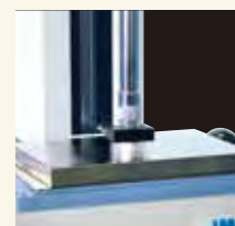
The test example of tablet strength test with PC-5060.
