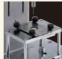
Film sticking test with TKS-250N
