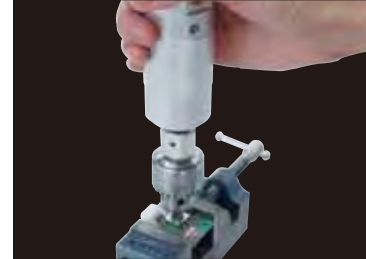
The test example of rotary switch click feeling test with HTGS.
