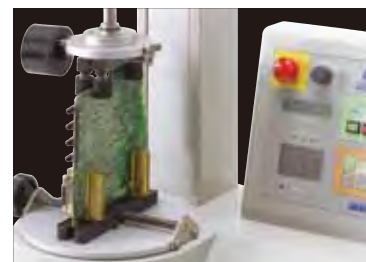
The test example of a circuit board twisting strength test with MTG.
