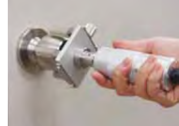
The test example of door knob turning force
