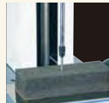
The test example of sponge hardness test with PG-2.
