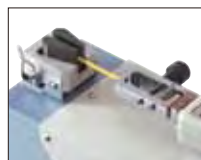
Test example of crimp contact strength test with LH-500N
