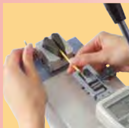
Only grip wire by lever operation
