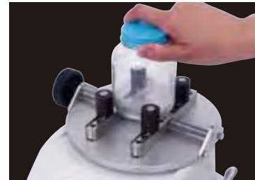
Screw cap opening torque test with DTXS.
