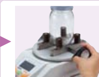
Turn the handle to fix the sample.
